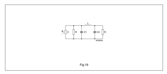
If C1 is the transistor output capacitance the components L and C2 must be added.
