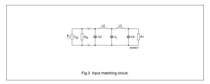
$C_i$  represents the input capacitance of the BLF245 which is appr. 220 pF (see Fig.6). Across this capacitor a constant voltage versus frequency from 25 up to 110 MHz has to be developed. Provided Ci is an ideal capacitance the optimum dimensioning of this network is as follows:
