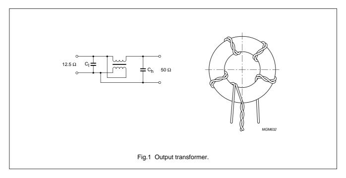
With the aid of a network analyser the transformer has been corrected for higher frequencies. With  $C_I$  = 68 pF and  $C_h$  = 12 pF the return losses in the range 20 – 140 MHz are better than –30 dB (VSWR < 1.07). Optimization of the complete output circuit has been carried out by measuring the return losses at the output with the network analyser under swept condition (see Fig.2).
